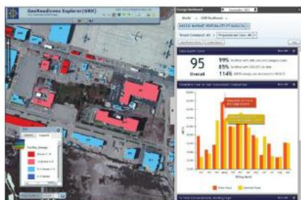
The Navy Shore Geospatial Energy Module (NSGEM) dashboard provides a bread crumb tracker and date picker to drill down to the geographic extent and lens for specific charts and reports. The map viewer renders buildings according to benchmark score, and the Data Quality Score highlights the accuracy and completeness of the information behind the dashboard.
